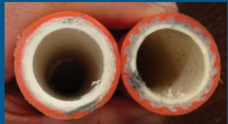
Fig.4 Old hose (left), and new hose (right) showing 'castellated' bonding with the outer skin
