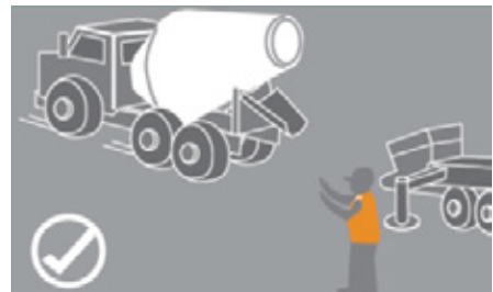
Keep clear when truck is reversing into position - ensure that you remain in the driver's view.
