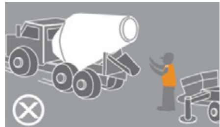
Keep clear when truck is reversing into position - don't stand between the truck and hopper.
