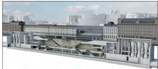
Figure 8. Paddington was a typical cut-and-cover 'box' station
