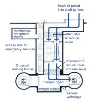
Section Through Ventilation Shaft
