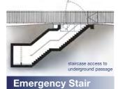
An access hatch beside Bayswater Road and a short subway to the shaft would give 24 hour access for emergency services to the staircase leading to the tunnels. The hatch would be flush with the grass behind the railings on Bayswater Road. A gate with a fire brigade lock would give access to the hatch.
