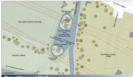
The proposed location for the ventilation shafts would be a strip of park between the existing Astroturf pitch and Garden Street. The narrow site would be away from the major open spaces of the park and partly concealed by existing mesh fencing. Garden Street would be closed to traffic and could become a new pedestrian route for the park. Nearby paths would be replanned around the site.
