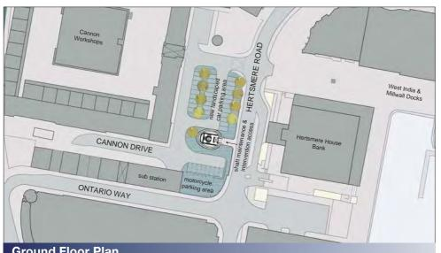
The shaft would allow access and emergency intervention to the tunnels below. As part of the shaft development, the existing car park could be rearranged to provide more car spaces than at present, possibly as indicated left.
