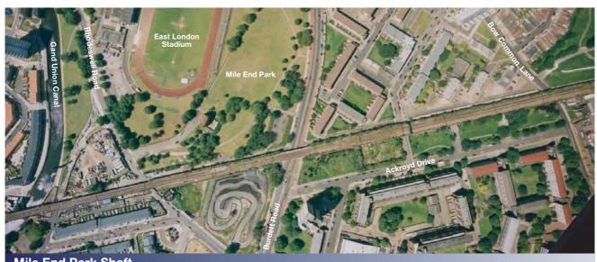
Mile End Park Shaft Intermediate shafts are required where there are distances of more than 1km between stations.
