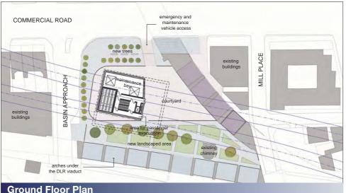
The shaft has been designed to provide tunnel ventilation, intervention and evacuation. The shaft would include a courtyard for maintenance and emergency vehicles. Vehicle access would be directly off Commercial Road through a gated enclosure. Separate site access would be provided to enable evacuation from the tunnels.
