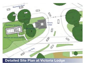
The shaft would contain a staircase and three fans. These would be switched on as required to assist tunnel ventilation or control smoke in an emergency. In either case, only two fans would be needed to operate at any given time, the third being a backup for maintenance. Sound absorbent material would be fitted to reduce operating noise.
