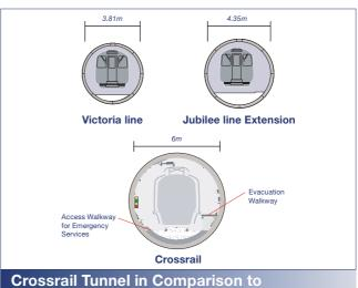
Crossrail Tunnel in Comparison to Existing London Underground Tunnels
