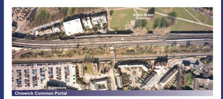
Crossrail proposes a tunnel from the Great Western Main Line near Ladbroke Grove to a portal at Chiswick Common. A station is proposed at Turnham Green to provide interchange with London Underground services.
