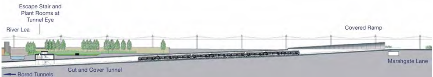
Proposed Pudding Mill Lane Portal – Section
