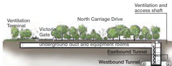
Duct and Shaft Section Looking North
