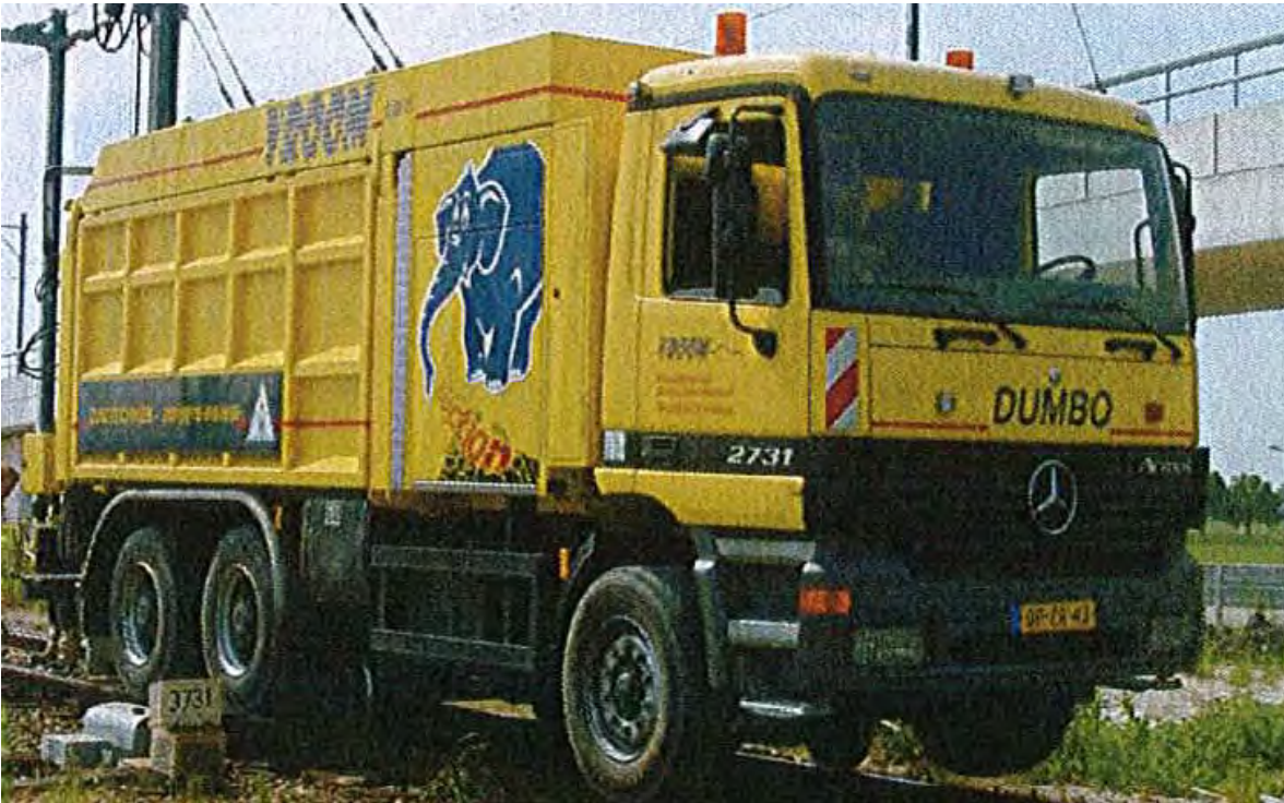
Figure 3: Madvac suction excavator of the type operated by Group 3.
