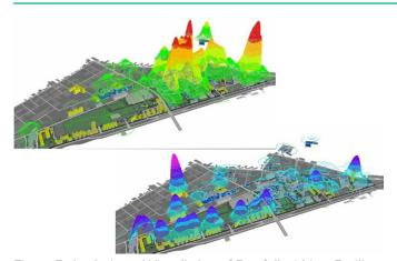
Figure 7: Analysis and Visualistion of Footfall within a Facility As a final example GIS can be used to undertake volumetric spatial analysis, allowing the planner or analyst to calculate the volume of air in the station, which in turn can assist with design or air filtration and cooling systems or calculate speed and direction of spread of fire or other hazardous incidents.
