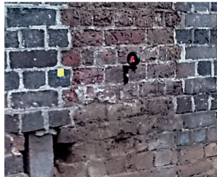
b) Prism on building facade – part of automated monitoring installation using Automated Total Stations
