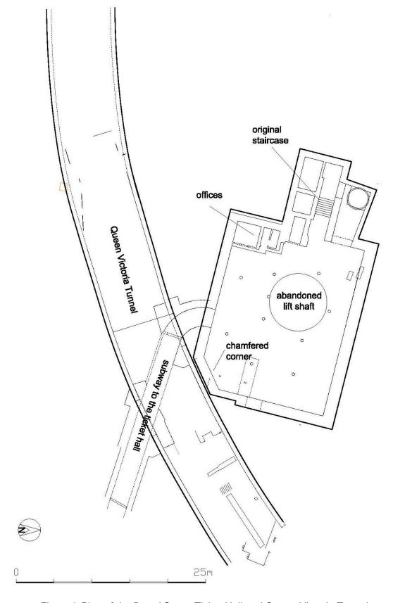
Figure 2 Plan of the Broad Street Ticket Hall and Queen Victoria Tunnel
