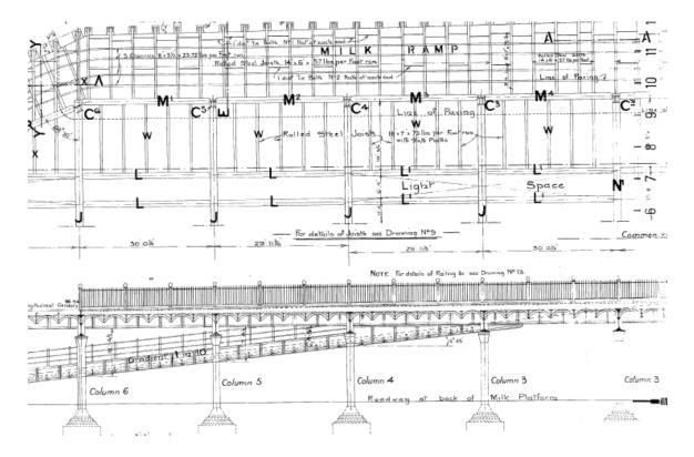
Plate F: Plan and section of London Street Deck showing milk ramp
