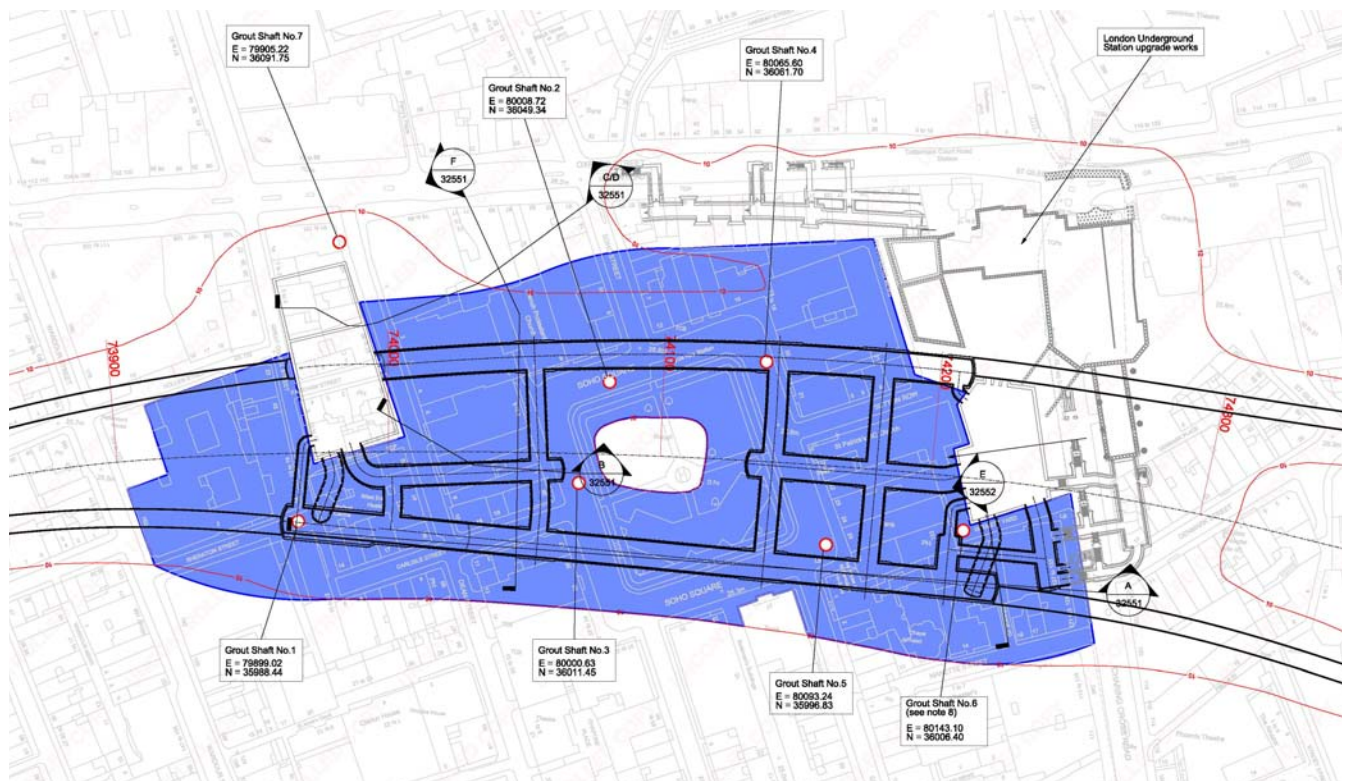
Figure 10: Proposed Grout Shafts at TCR
