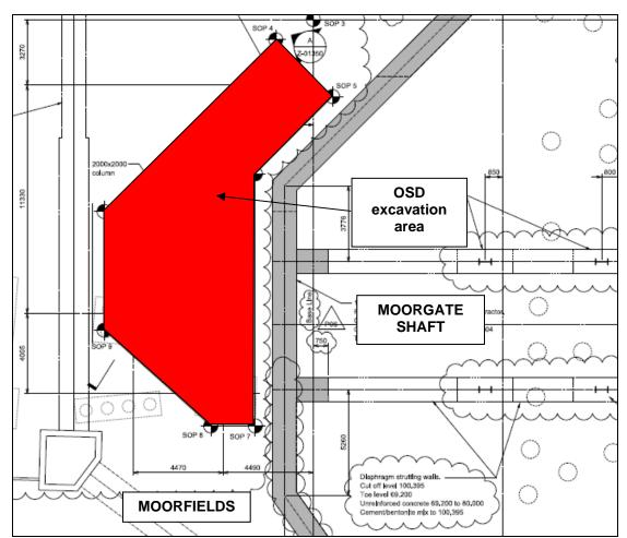
Figure 4 OSD foundation excavation area
