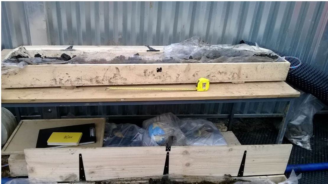
Photo 3 Column sample from borehole, laid out ready to be inspected
