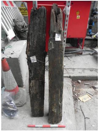
Photo 10 Manhole S4, 19th-century timber shoring, after excavation
