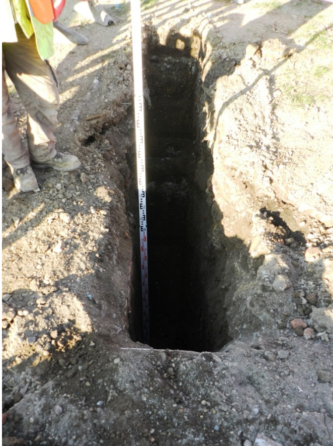
Photo 1 Coal-ashy fills in TP1 looking north
