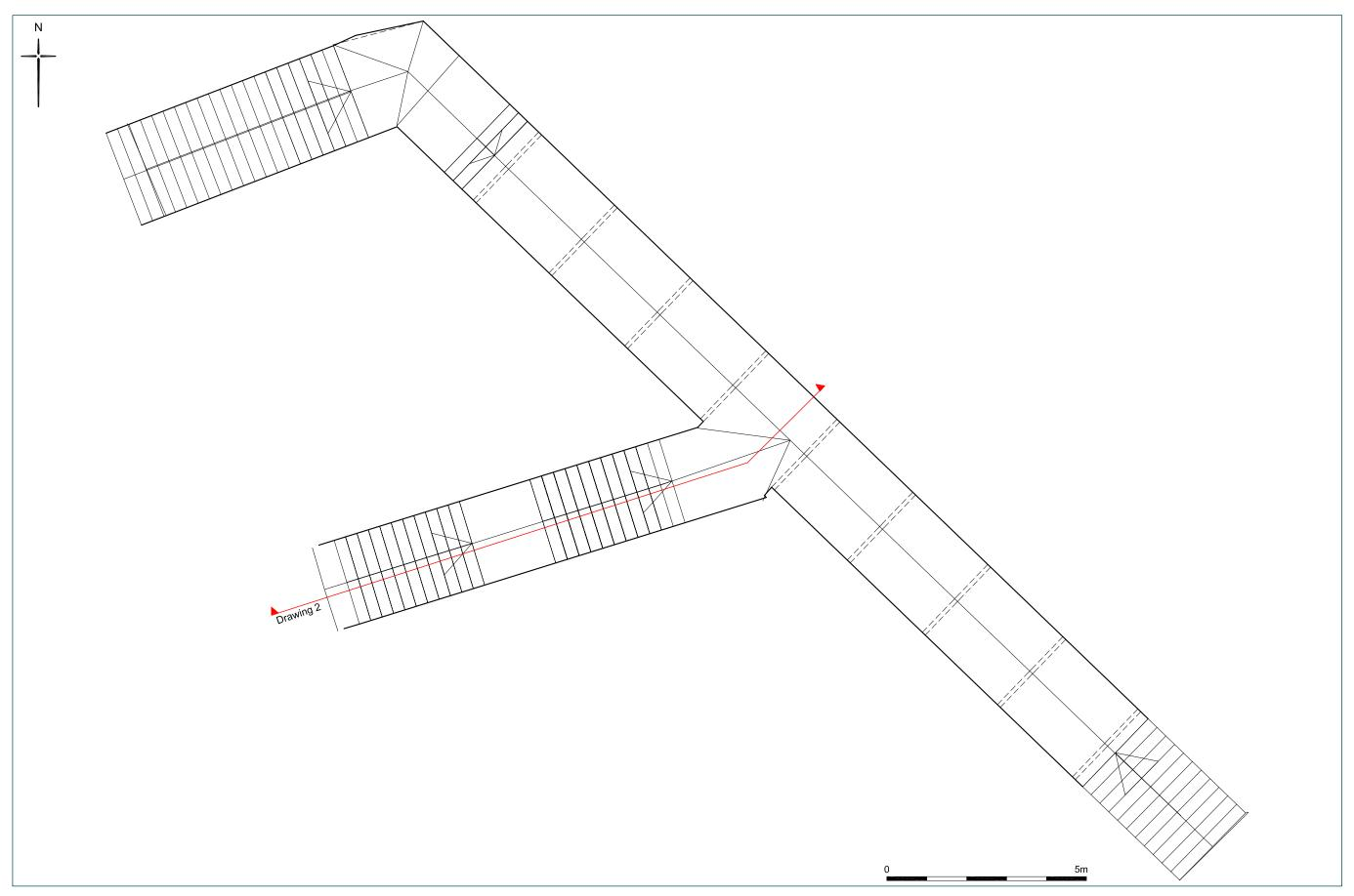
Drawing 1 plan of Item 2, the footbridge and step-stairs to the platforms
