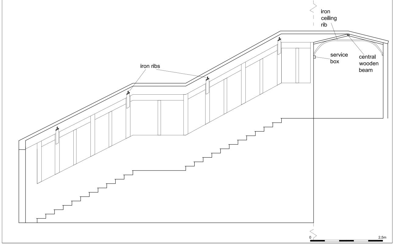
Drawing 2 Longitudinal sectional view of the staircase from the footbridge to platform 1 and 2 and cross section of the footbridge (looking north).
