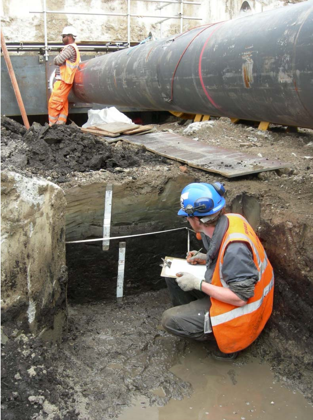
Photo 6, Sampling the sequence through the upper alluvium [4], peat [5] and underlying gravels [6] in Trench 1D (looking northeast).
