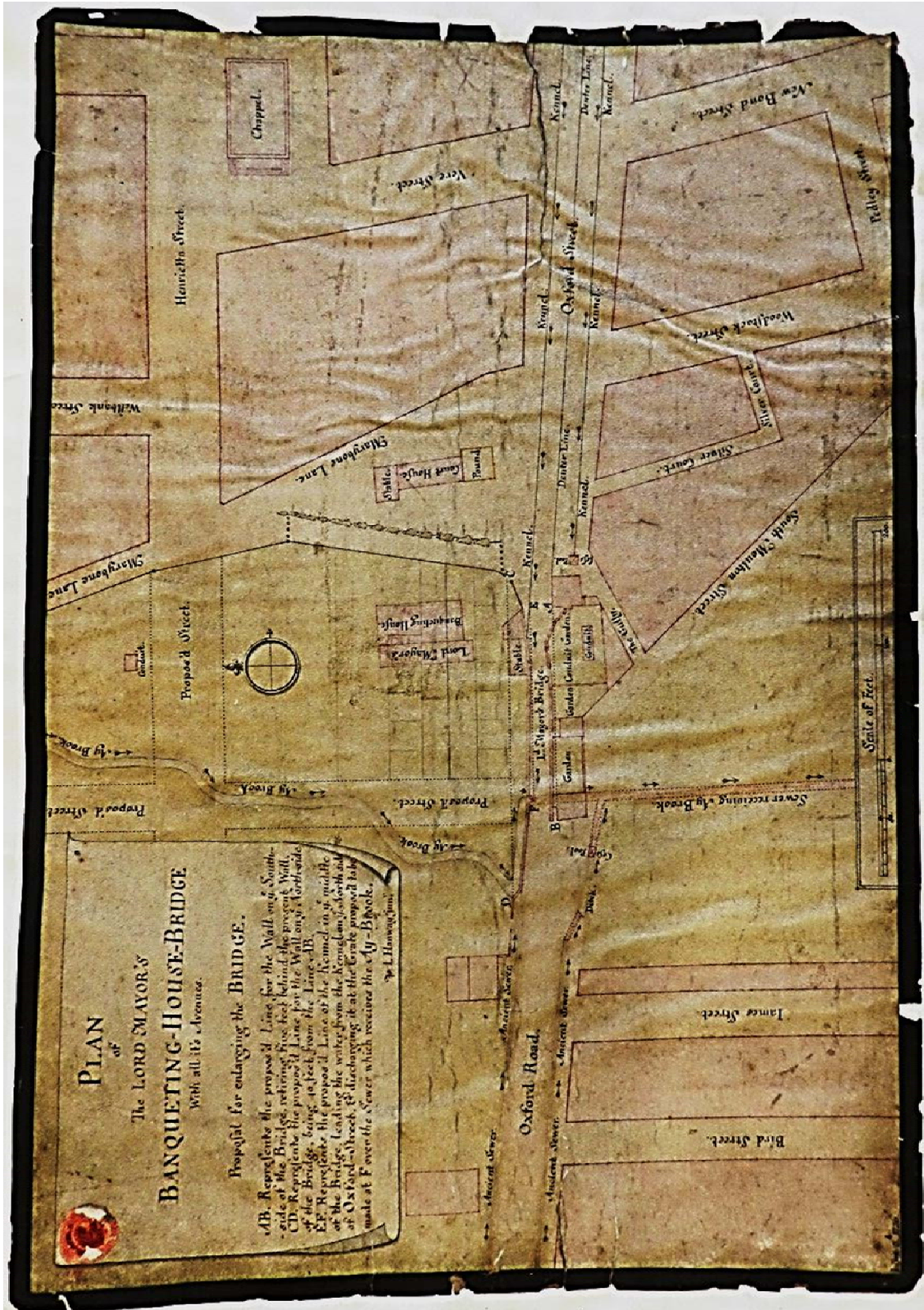
Fig 28 A plan of the lord mayor's banqueting house bridge with enlargement proposed (Westminster Archives)
