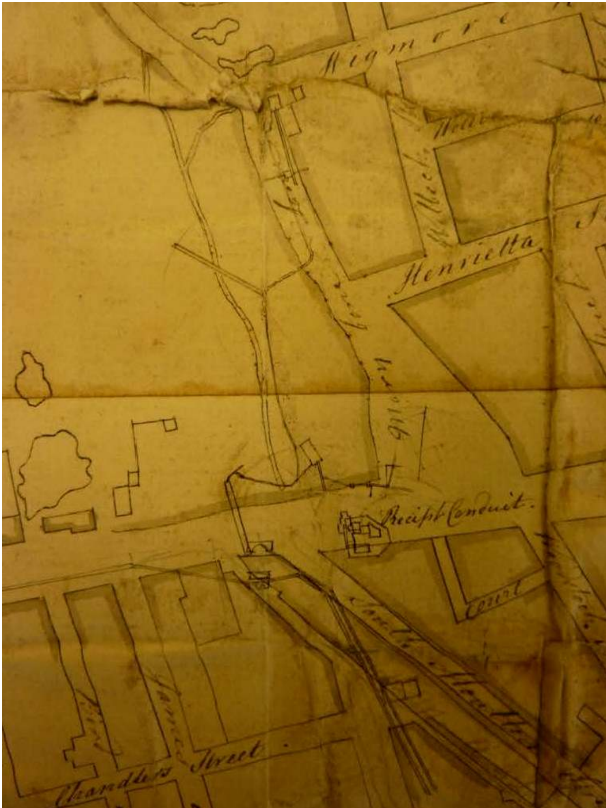
Fig 26 A post 1737 plan to re-route the conduits and create an aqueduct passing along Marylebone Lane
