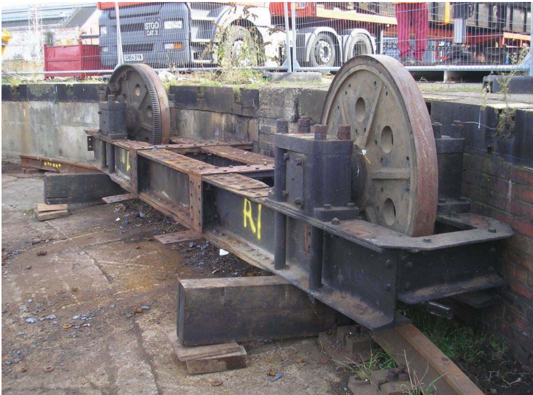
Plate 58. 'Manual' drive bogie after turntable lifted off.
