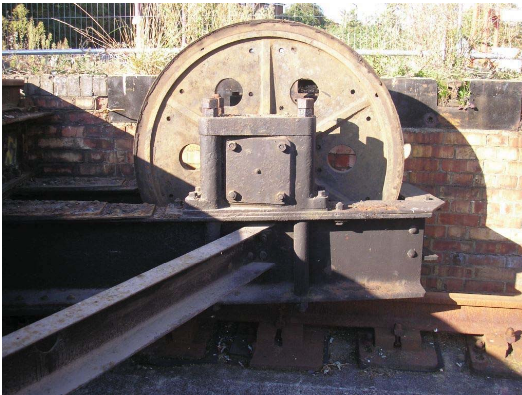
Plate 38. Free wheel at hand crank end with diagonal bracing beam to bogie and steel rim to iron wheel. the
