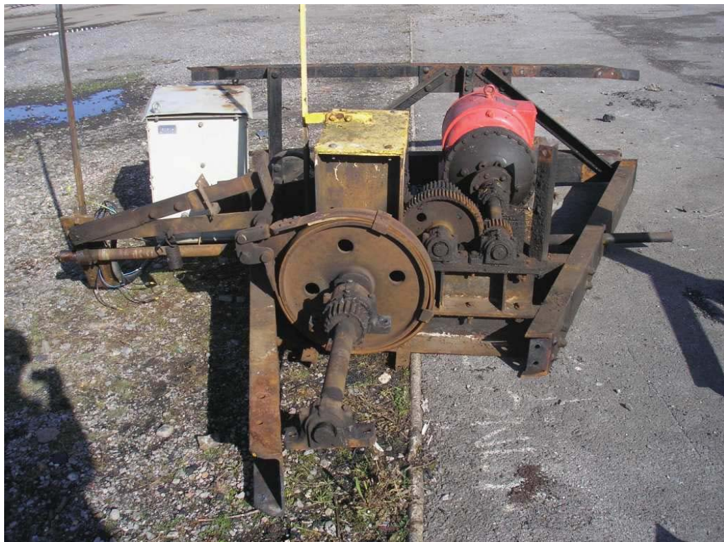
Plate 44. Electric drive unit with circular brake disc on drive shaft in foreground.
