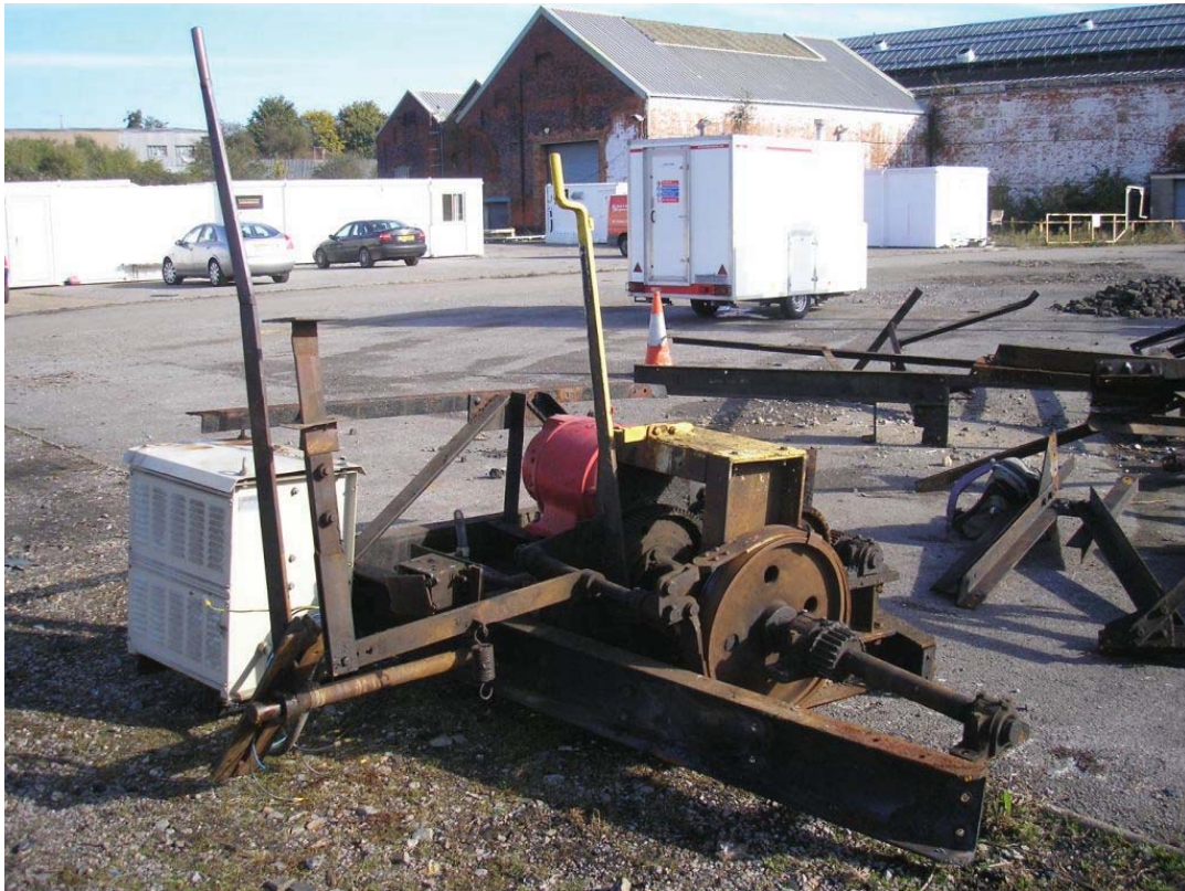
Plate 43. Electric drive unit and transformer in white casing. On the left is the locking bolt lever, brake pedal and the centrally located manual/electric operation lever.
