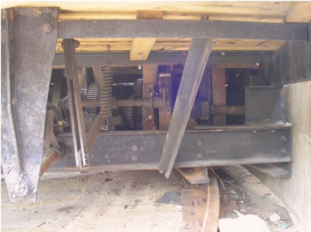
Plate 27. Side-on view of electrically powered drive mechanism and turntable wheel.
