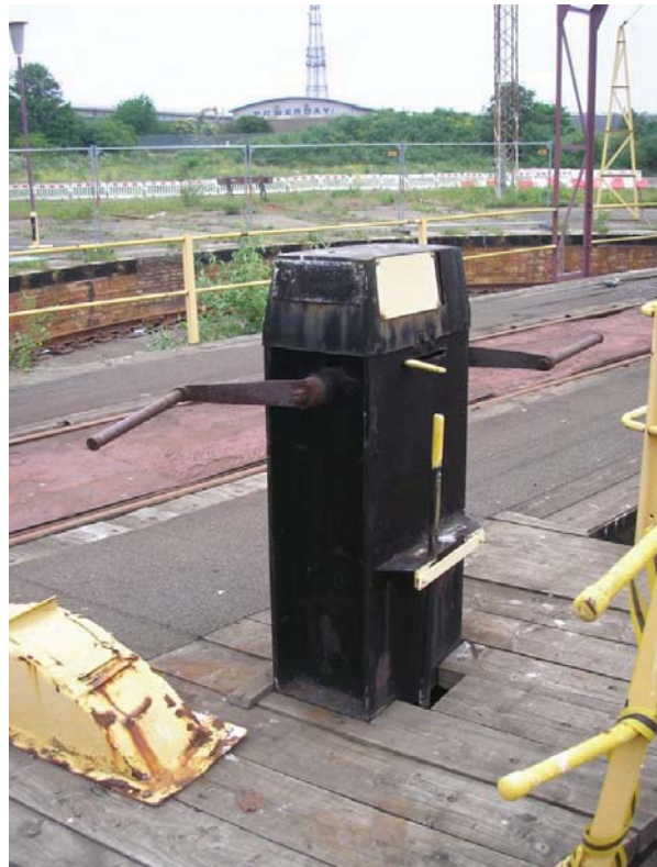
Plate 16. Hand crank mechanism with horizontal reverse lever and vertical manual/electric operation lever.
