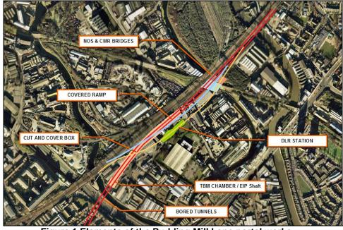
Figure 1 Elements of the Pudding Mill Lane portal works
