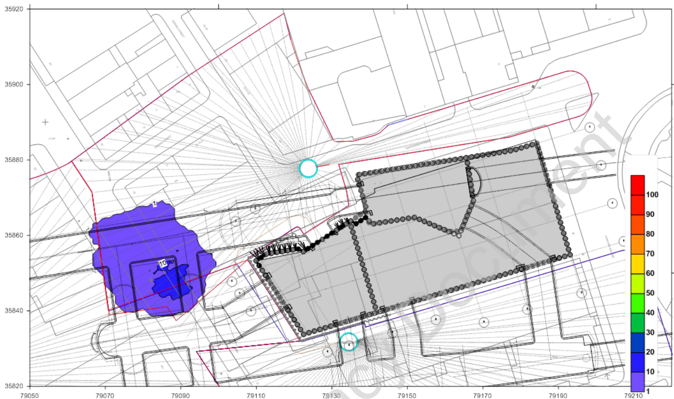
Figure 3.6.4 Period E: Distribution of grout injected from GS3: Grout jacking ( l/m^2 ).
