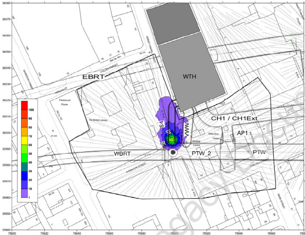
Figure 3.6.3 Period E: Distribution of grout injected from TCR GS1: Grout jacking. Grout Intensity (mm).
