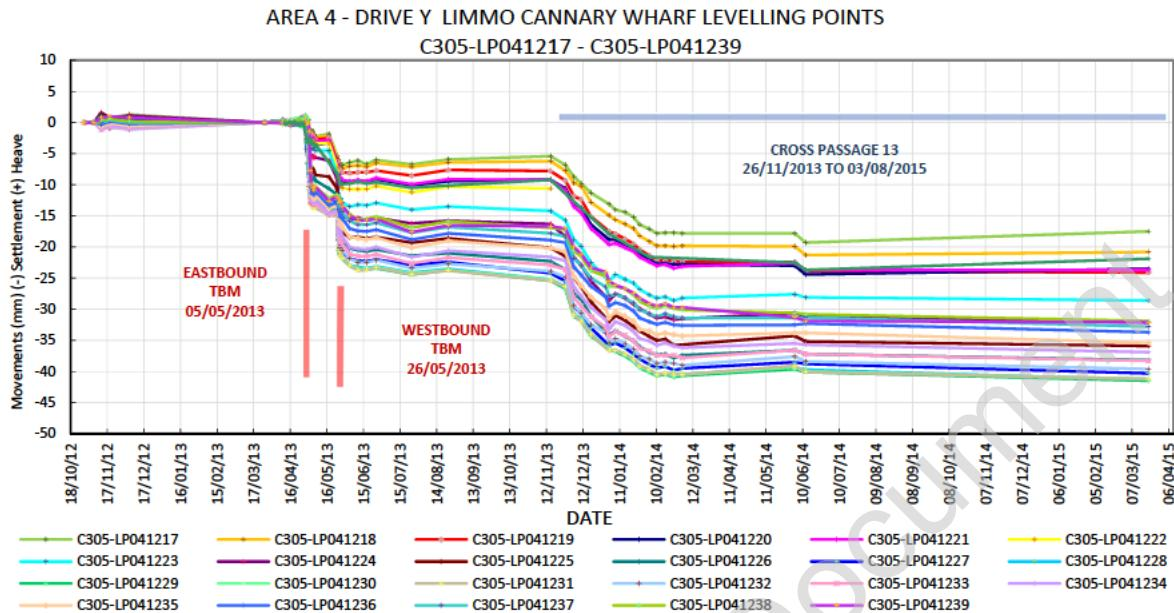
The graph above shows a maximum settlement of -12.3 mm after the eastbound TBM transit and a total maximum settlement of -21.5 mm after the westbound TBM transit. The total maximum settlement due to dewatering in Cross Passage 13 is -41.2 mm.
