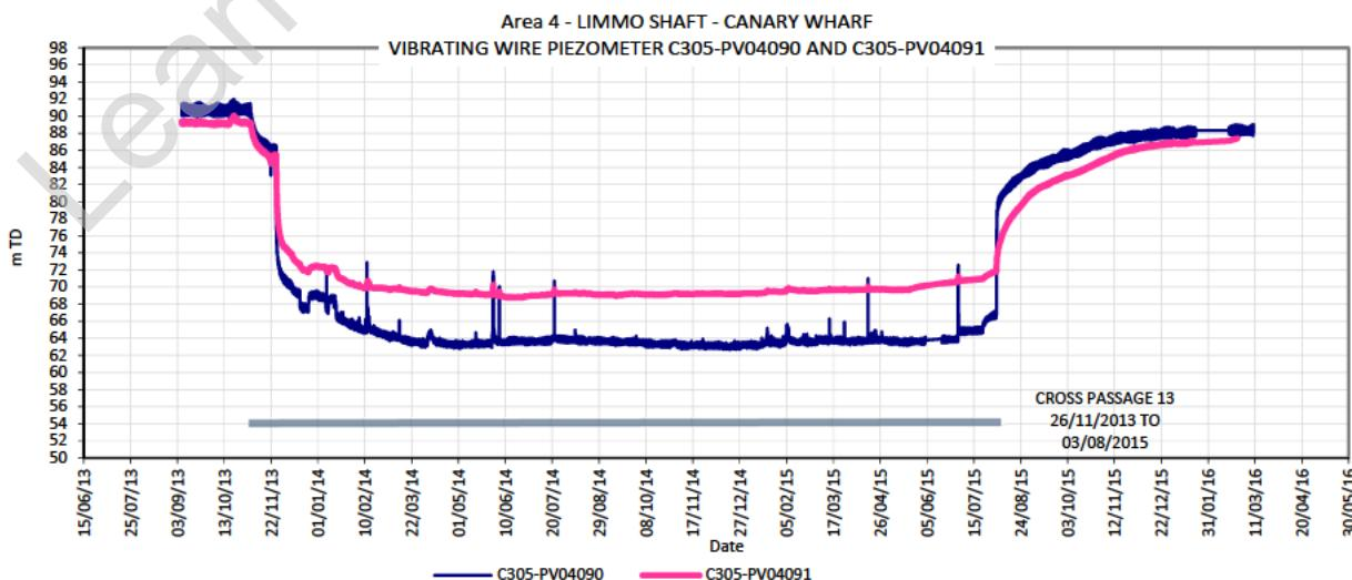
Note: The depth of the response zone of C305-PV04090 is located in Chalk at 59.5 m and C305-PV04091 is located in Sand at 47.5 m.
