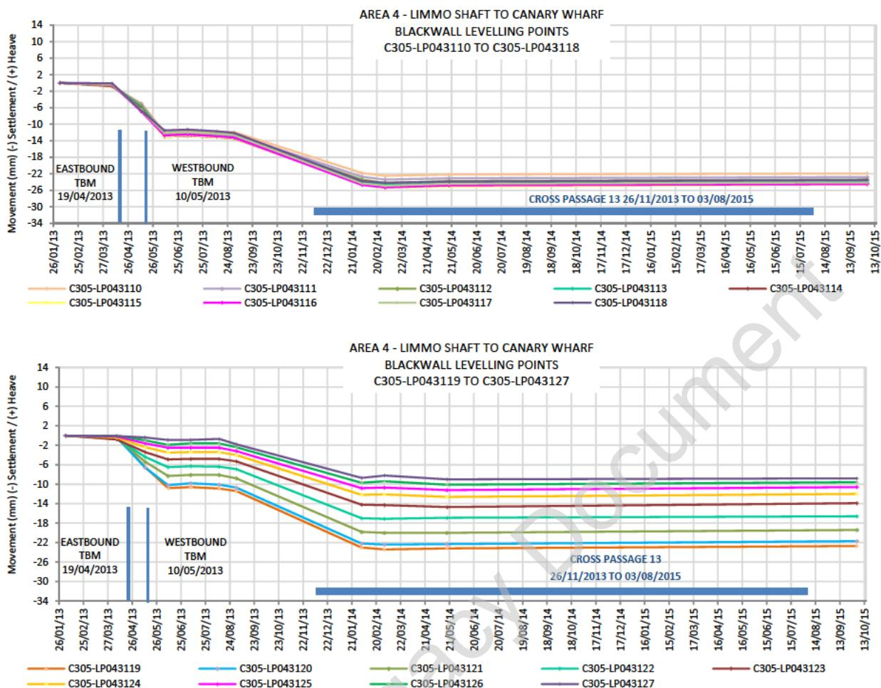
In order to determine if the rate of change in the data has reached an acceptably small rate, the last two readings (this includes one reading after the dewatering period) were used to calculate the annual projection.
