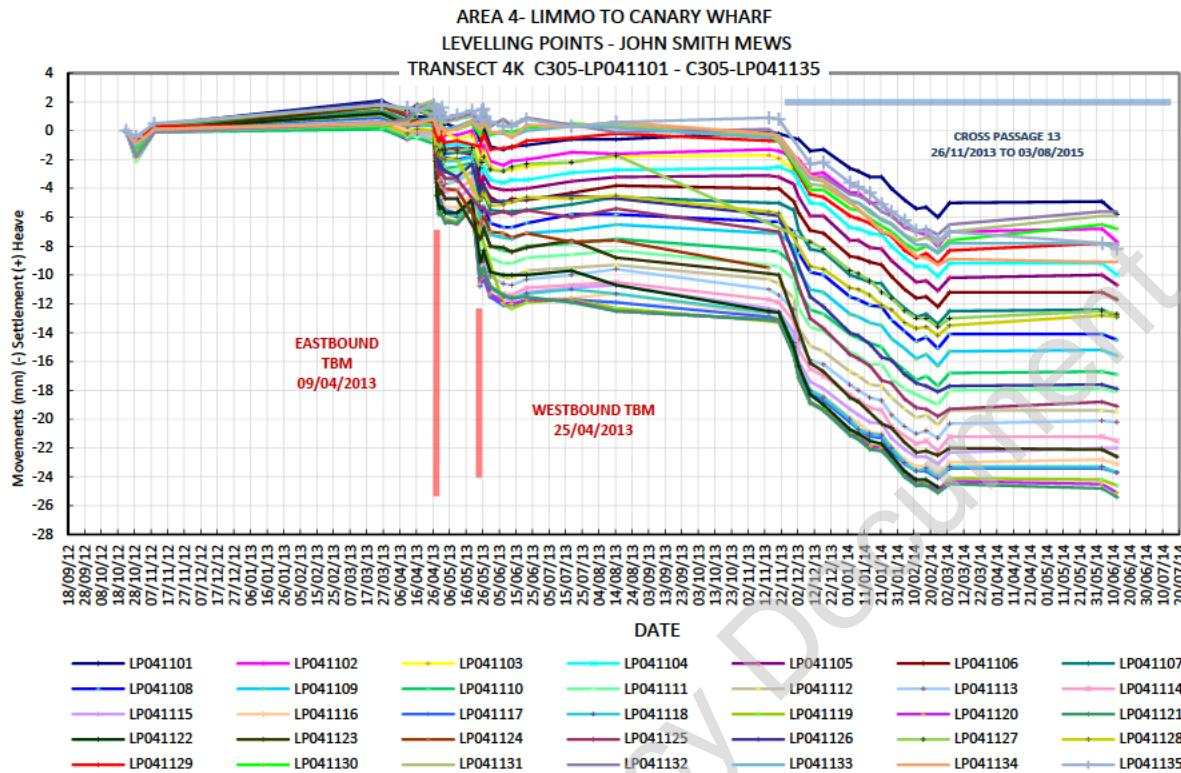
The graph above shows a maximum settlement of -6.4 mm after the eastbound TBM transit and a total maximum settlement of -12.3 mm after the westbound TBM transit. The total maximum settlement due to dewatering in Cross Passage 13 is -25.4 mm.
