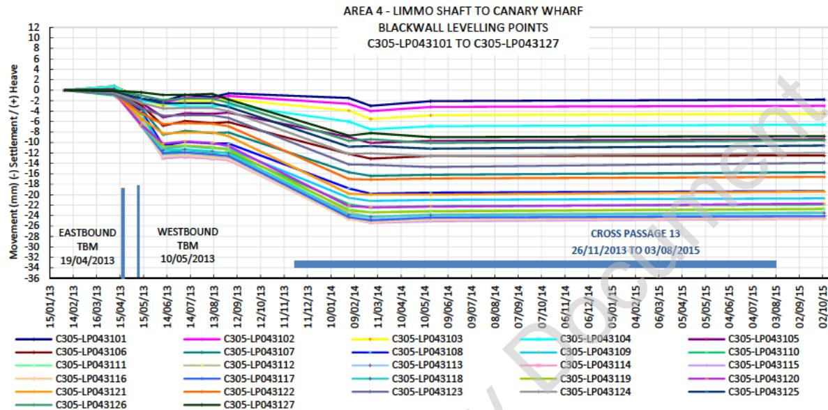
The following graphs presented below are from different sections of the leveling points array installed within the Blackwall northbound tunnel.
