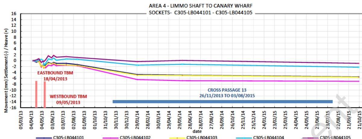
The graph above shows a maximum settlement of -2mm after the westbound TBM transit, and a total maximum settlement of -7mm during the dewatering period of Cross Passage 13.
