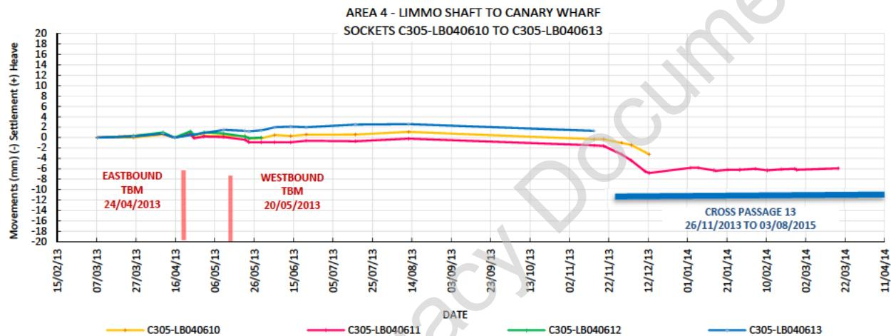
No projection has been calculated for this array because some of the sockets were damaged/destroyed and no further readings were taken after the dewatering of Cross Passage 13.
