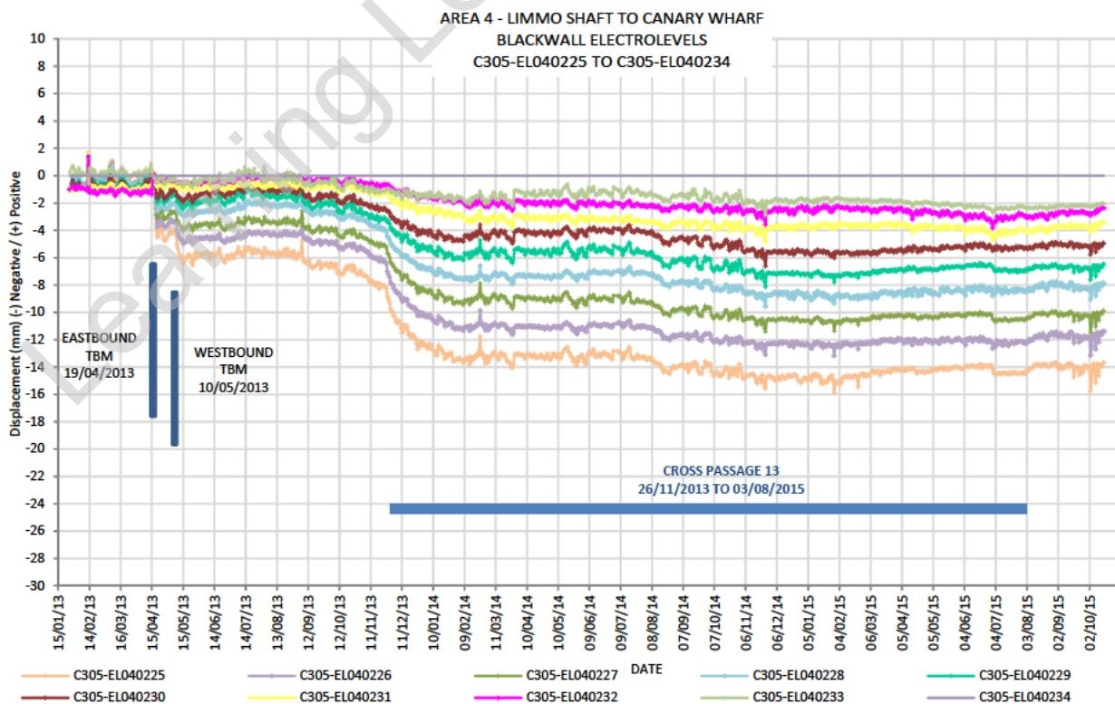
The graph above shows data recorded from electrolevels located along the north section of the line. There was -4.7mm settlement after the eastbound TBM transit and a total maximum settlement of -6mm after the westbound TBM transit. The dewatering of CP13 shows a total maximum settlement of -15mm.
