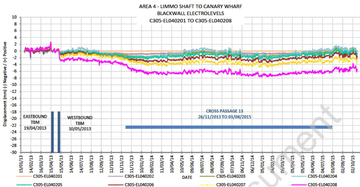
The graph above shows data recorded from the electrolevels located in the south part of the electrolevel line; there was no significant movement after the eastbound TBM transit and a maximum settlement of -3mm after the westbound TBM transit. The dewatering of CP13 shows a maximum settlement of -8mm.
