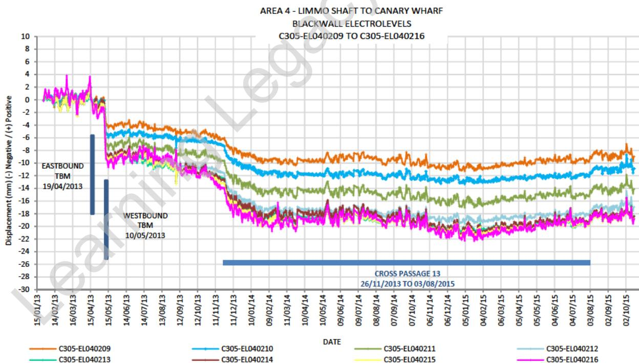
The graph above shows data recorded from electrolevels located above the westbound tunnel alignment. There was -2.9mm settlement after the eastbound TBM transit and a total maximum settlement of -11mm after the westbound TBM transit. The dewatering of CP13 shows a total maximum settlement of -22mm.
