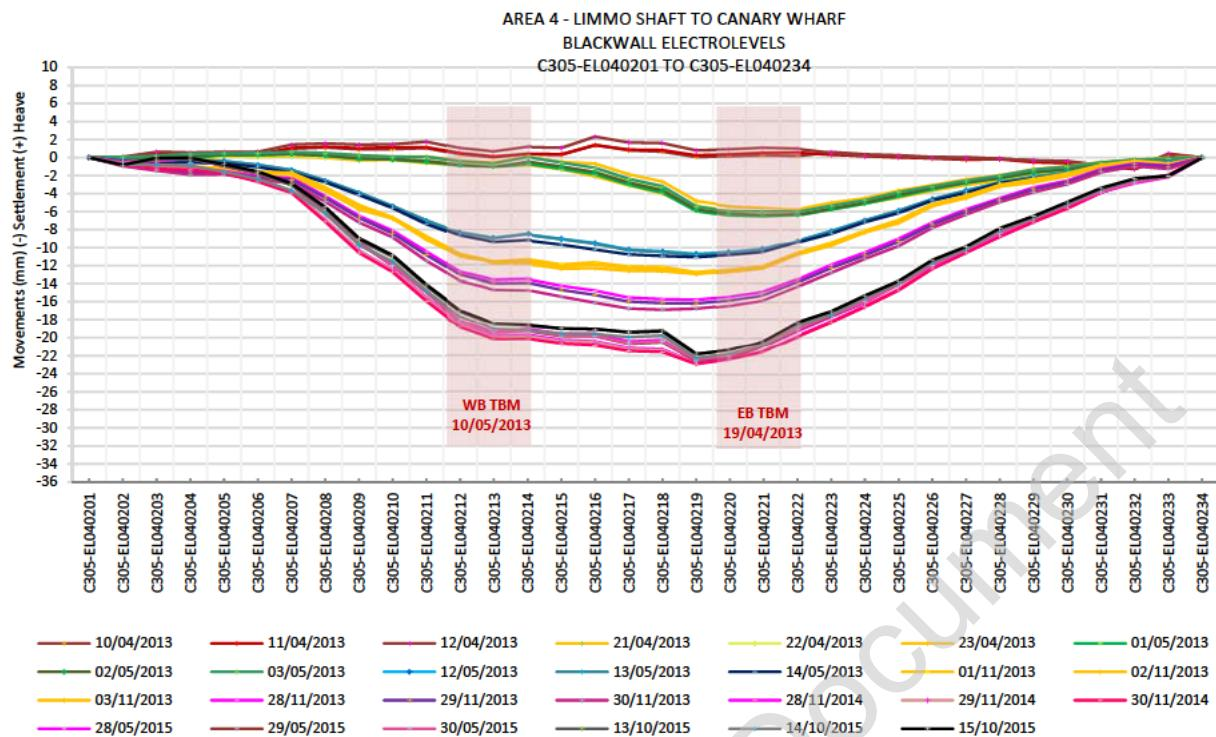
The graph above shows a settlement of -6mm after the eastbound TBM transit (for electrolevels: C305-EL040220 to C305-EL040222). After the westbound TBM transit, the total maximum settlement was -10mm (for the electrolevels: C305-EL040212 to C305-EL040214. The dewatering period for Cross Passage 13 shows a total maximum settlement of -23mm.
