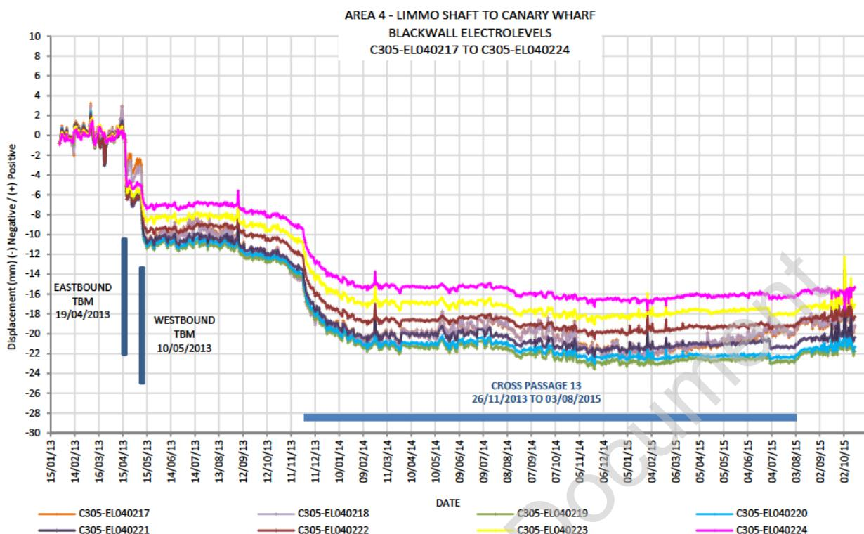
The graph above shows data recorded from electrolevels located above the eastbound tunnel. There was -6.7mm settlement after the eastbound TBM transit and a total maximum settlement of -11mm after the westbound TBM transit. The dewatering of CP13 shows a total maximum settlement of -23mm.
